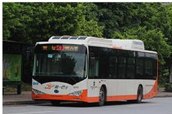
The BYD electric bus or BYD ebus, called K9 in China, is an all-electric bus model manufactured by Chinese automaker BYD, powered with its self-developed Iron-phosphate battery, allegedly featuring the longest drive range of 250 km (155 miles) on one single charge under urban road conditions.
